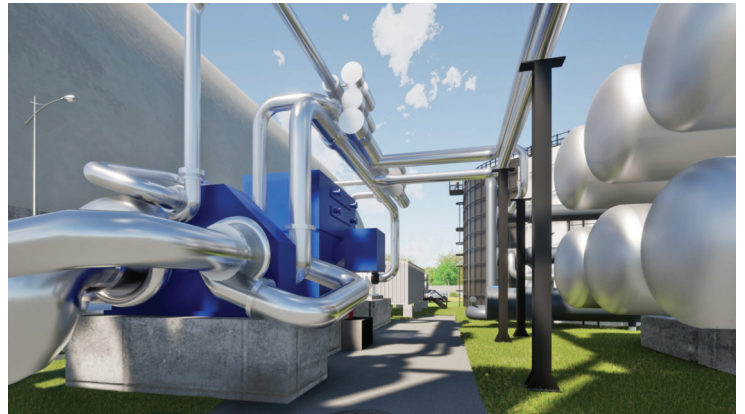
Close-up of CO 2 battery
