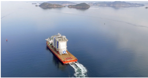
The HSRGs modules were barged from Tongyeong-si at the Goi site
