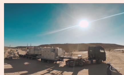
Trailer-mounted TM2500 gas turbine
