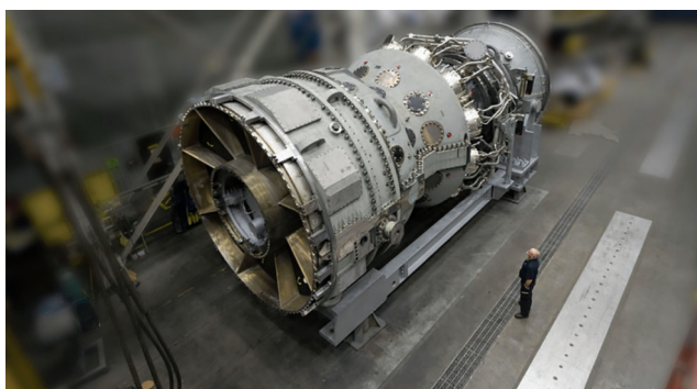
7HA.03 gas turbine
