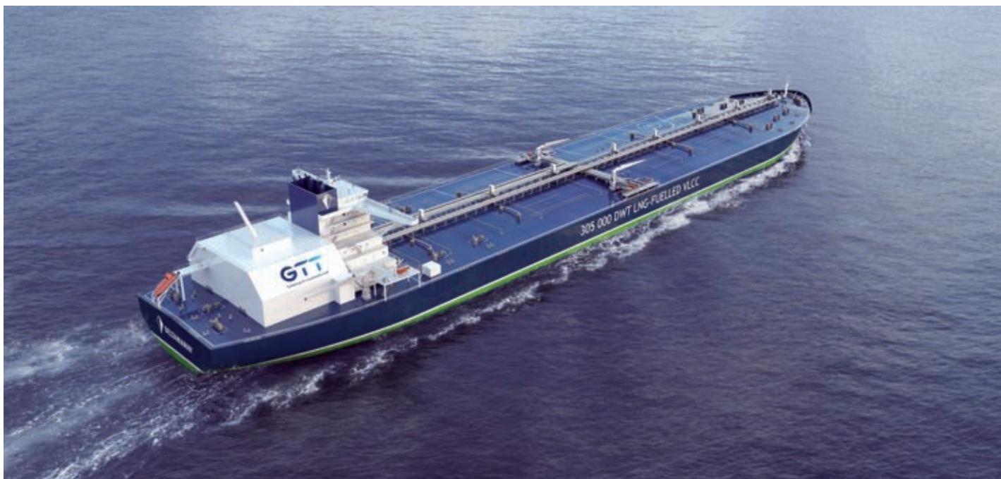
One of the latest examples of an LNG fuelled ship design is this 305,000 dwt VLCC put forward by Deltamarin and GTT, which has recently been awarded an AIP by ClassNK
