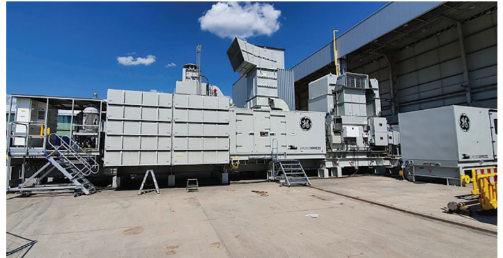
Trailer-mounted LM2500XPRESS gas turbine
