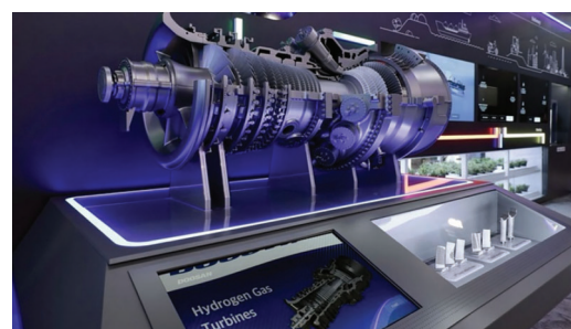
Model of Doosan's 380 MW hydrogen gas turbine
