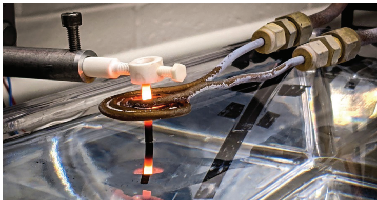
3D-printed superalloy drawn through an induction coil
