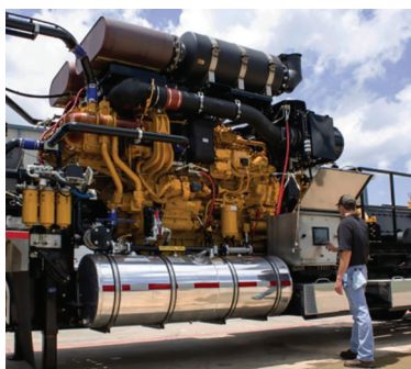
Cat 3512E Tier 4 dynamic gas blending engine
