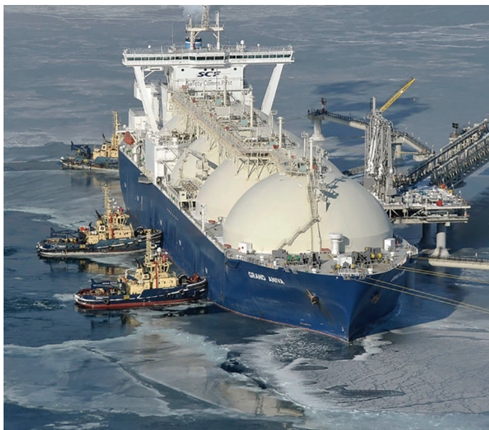
An LNGC seen at a Sakhalin-2 loading berth
