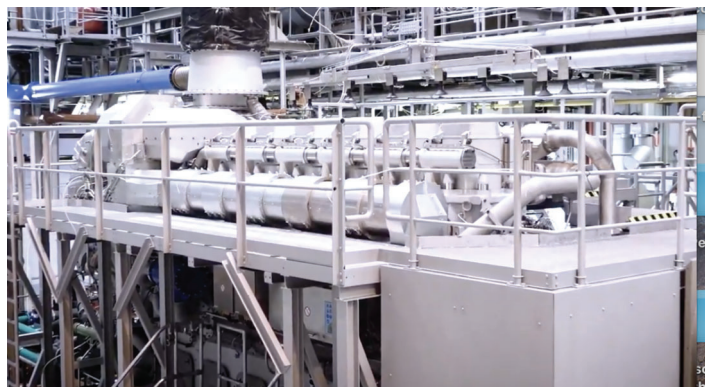
Dual-fuel electric propulsion proposal based on 49/60DF engine from German firm MAN Energy Solutions
