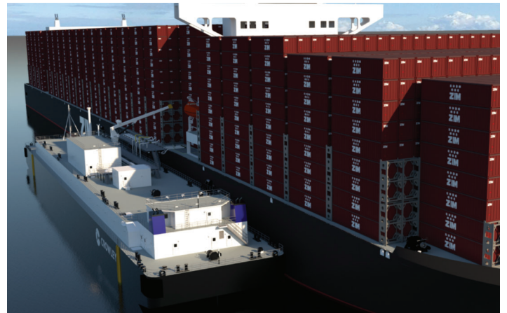
Graphic of the 12,000 cubic metres capacity bunker barge
