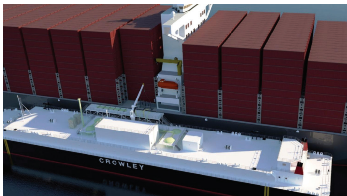
Bunker barge during refuelling
