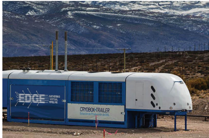
Truck-delivered LNG equipment includes two Cryobox technology units and can monetize stranded gas
