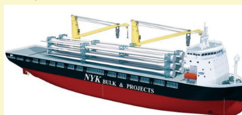
NYK's new heavy lift ships will be able to lift LNG plant equipment
