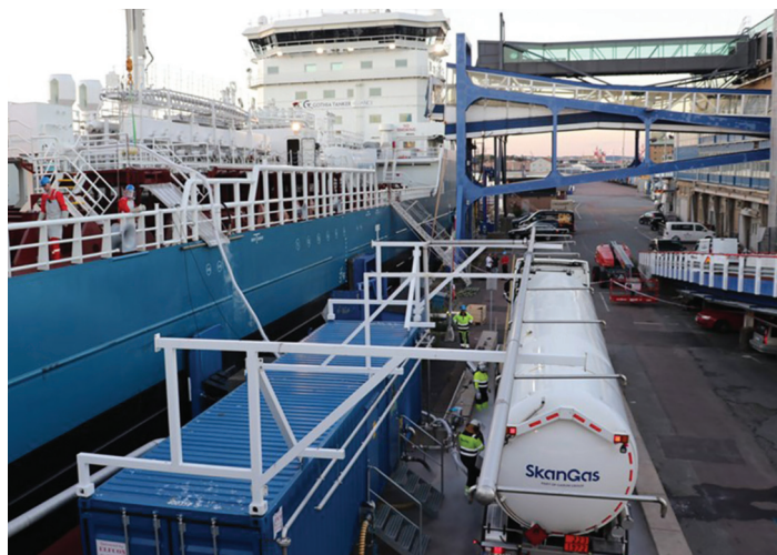
Fure Vinga refuels with liquefied biogas
