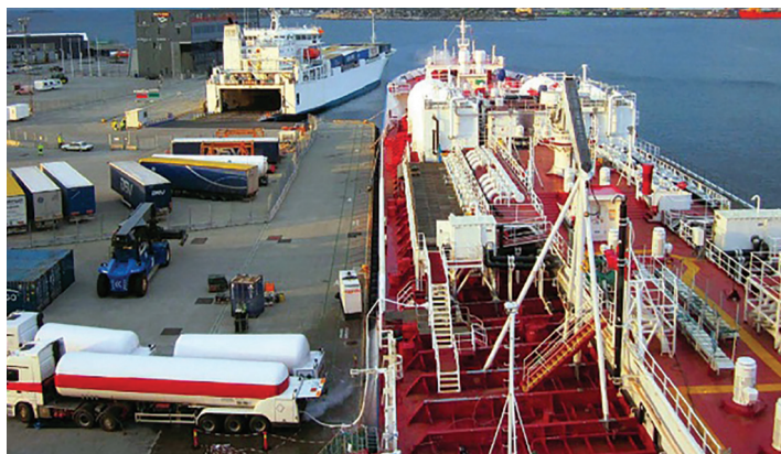
Vessel refuels with LNG in Singapore
