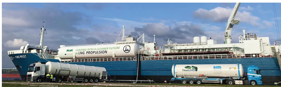
Titan LNG trucks during refuelling operations
