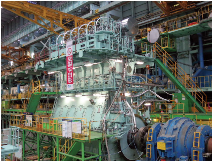
The LNGC is fitted with two of the new WinGD 6X62DF dual fuel engines
