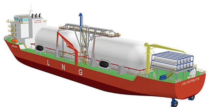
Wison has designed an LNG distributor vessel, which can be built with a capacity of between 5,000 and 20,000 cu m
