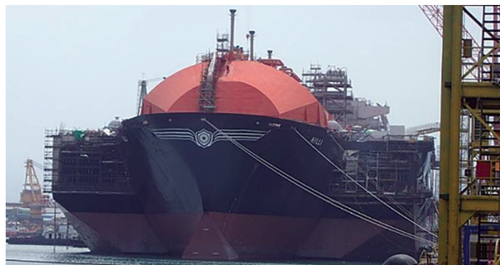
LNG carrier 'Hilli' under conversion at Keppel in Singapore
