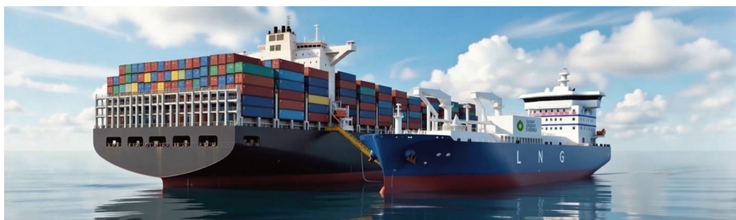
Mistral LNG during bunkering
