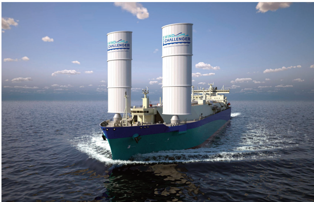
A rendering of the wind sails fitted on an LNGC
