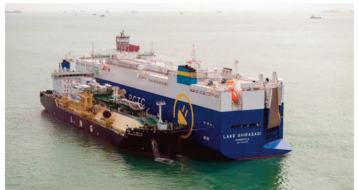
FueLNG Venosa conducting STS bunkering
