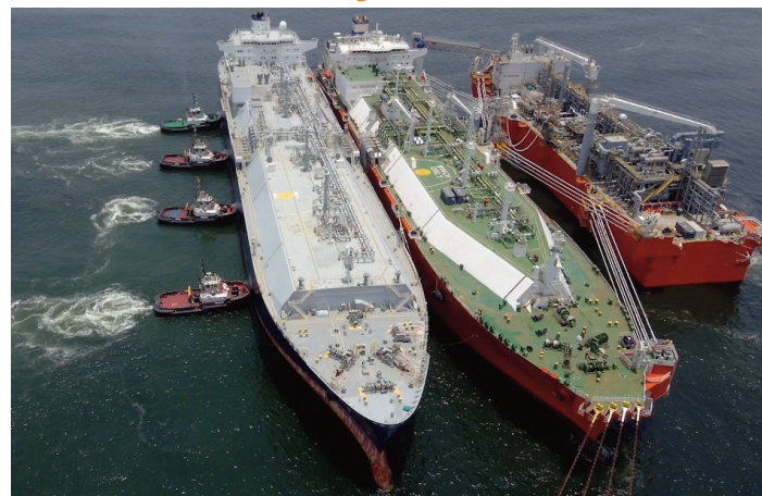
Configuration called 'split mooring' off the Congo coast
