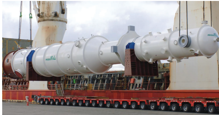
Air Products LNG equipment being loaded at Florida factory
